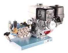
The pump sets with a fuel engine are in a standard manner manufactured with a Honda petrol engine, equipped with a minimum oil safety and repeated starter. Small capacity membrane pumps are directly driven by means of a reduction gear as a result of which they can be constructed in a very compact manner. The composition of the larger capacity and plunger pumps equals such of the pump sets with an electric engine.
